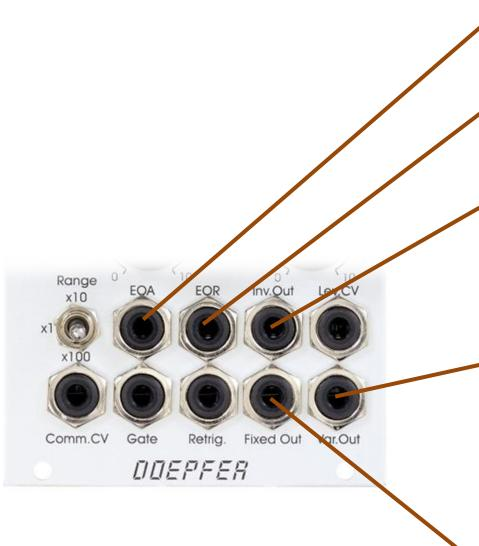
**EOA:** Gate output that emits a positive voltage as soon as the attack phase has ended. The gate signal ends at the start of the release phase.
