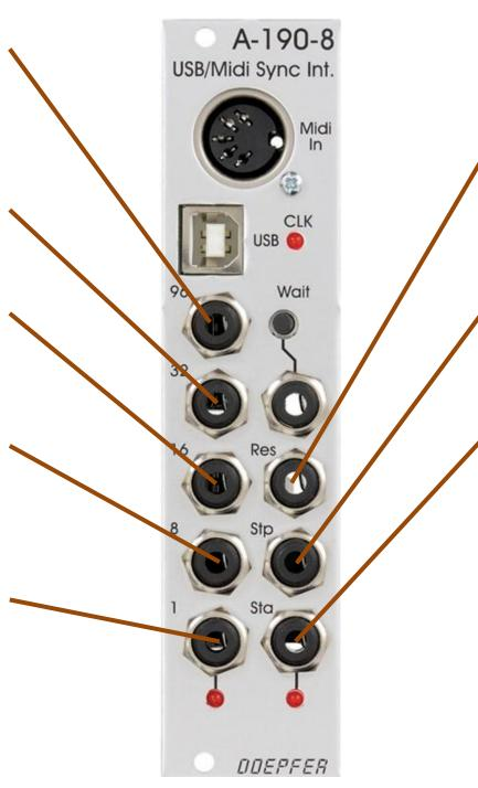
**Res:** As soon as a midi start signal follows a midi stop, a trigger to reset the (analogue) sequence is output here.
