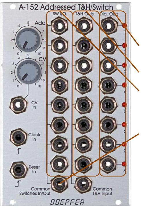
**Dig Outs 1 to 8:** Gate outputs that emit a gate signal when the level is active, 0V when the level is inactive.
